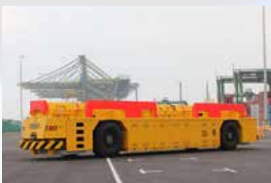
Yangshan Port, Shanghai Automated transfer vehicles at the world's largest automated wharf.
